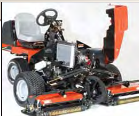
19hp ISO mounted diesel engine mounted between the front wheels offer low centre of gravity
