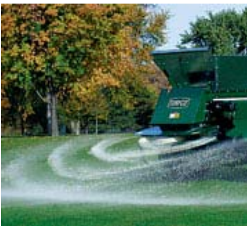
Adjustable twin spinners angle down for better penetration of turf.
